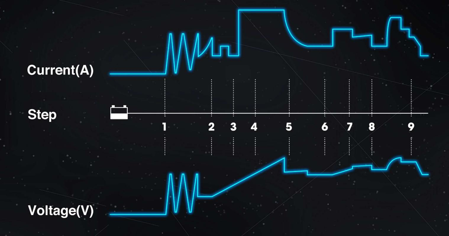
Its "9-step smart charging" provides strong protection to the battery and the automatic charging and disconnection system eliminates any risk of overcharging.
